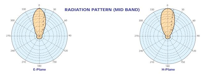
Gain is provided for vertical polarization.
