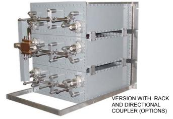
The star point combiner basically consist of parallel connecting several transmitters to a single antenna system through suitable band pass filters, each on tuned transmitter frequency to witch it's connected. The parallel connection is obtained by means of coaxial
